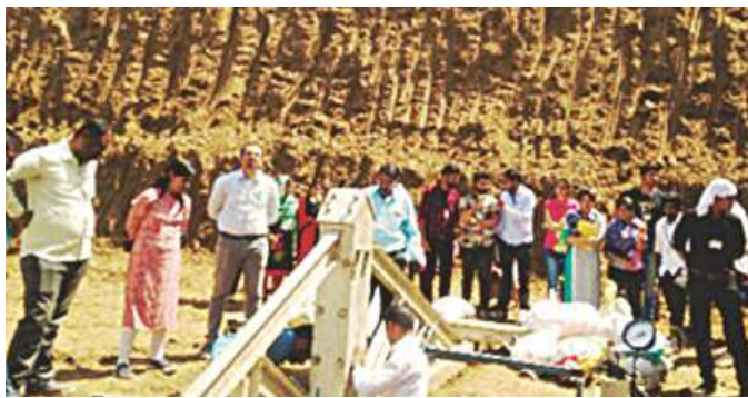
Plate Load Test by Civil deptSSBTCOET at TapiPatbandhareVikasMandalBodwad
